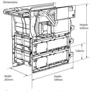
The dimensions above are based on a standard two denomination mechanism with 85mm throat extension. To calculate the dimensions for additional denominations add 128mm to the height.
