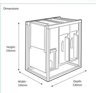
The dimensions above are based on a standard two denomination mechanism. To calculate the dimensions for additional denominations add 147mm to the depth.
